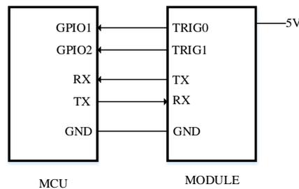
Figure 2. The connection between the P1220 and external device
